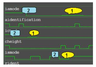
The signal (1) from the omnidirectional antenna is less that signal from directed antenna (2). This means that the captured aircraft flies in the main-lobe of the monopulse radar. Other segments of the signal originating from other aircrafts, which are not flying in the main-lobe, will not be processed as long as the radar antenna isn't directed to them.
