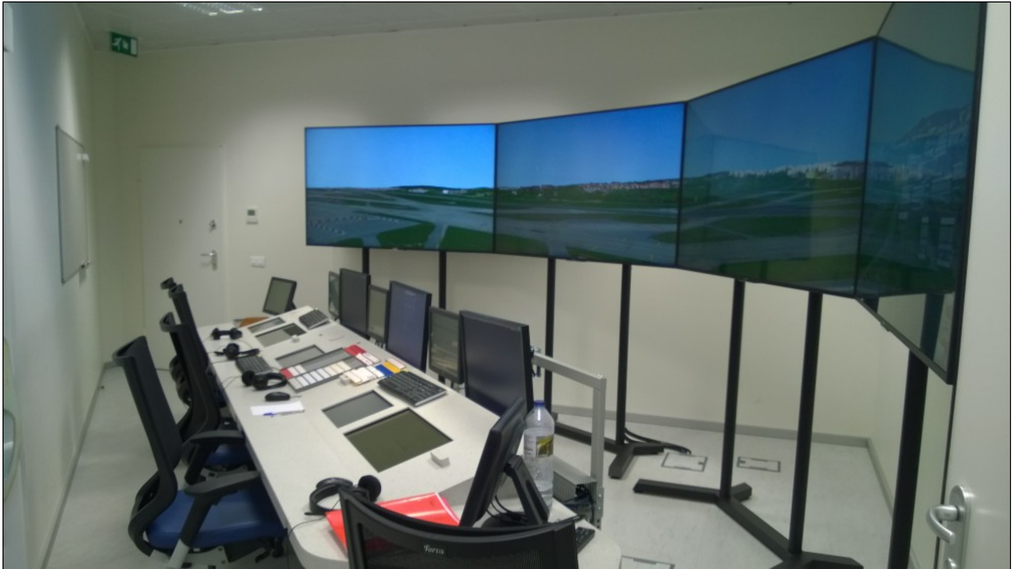
TWR Controllers Room - 4x large LCDs 75", 200 degrees view
