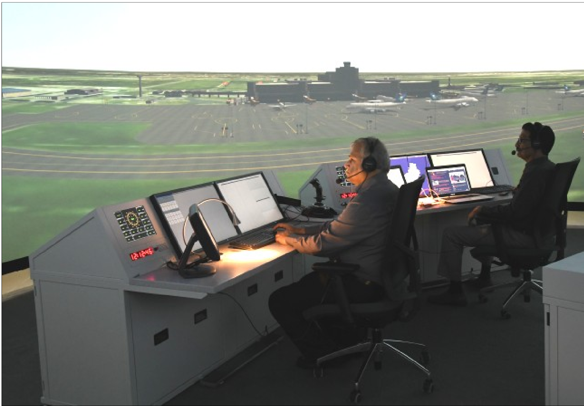
360 degrees projection TWR Sim dome
