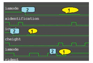
The signal (1) from omnidirectional antenna is less that signal from directed antenna (2). This means that the captured aircraft flies in the mainlobe of monopulse radar. Other segments of the signal originating from other aircrafts, which are not flying in the mainlobe will not be processed as long as the radar antenna isn't directed to them.
